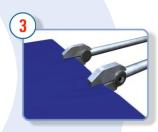
Gripper arms: Incorrectly adjusted high pressure gripper arms can break and tear the edges of PLPs.
