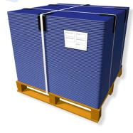
Return delivery conditions: PLPs should be stacked to a height of approximately 90 cm, secured with either a shrink bag, stretch film or plastic straps and labeled with a pallet identification tag.
