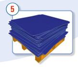
Incorrect stacking: Manual stacking without a frame allows PLPs to slide over each other creating an irregular stack and increasing the risk of damage.
